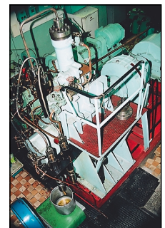
Experimental Plants for testing high pressure fuel equipment of low-speed engines MAN B&W
