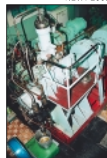
Experimental Plants for testing high pressure fuel equipment of low-speed engines MAN B&W
